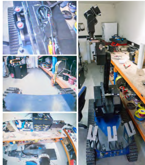
Fig. 6. The tEODor robot navigating a particularly tight environment, in this case a gap with approximately 3 cm of clearance to either side of the robot. The views from the standard cameras are shown left top and centre. The view from the wide angle camera is shown to the bottom left.
