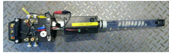
Fig. 8. The new camera probe, compatible with the tEODor's tool changing mechanism and housing two cameras, one pointing out of the end and one pointing sideways.
