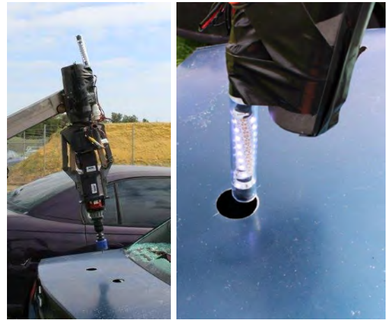
Fig. 4. Flexible probe consisting of a wide angle camera and LED lamp attached to the back of the tEODor's gripper. This allows the gripper to be used as normal, such as to hold and use a drill (left) and then turned around to deploy the probe (right).
