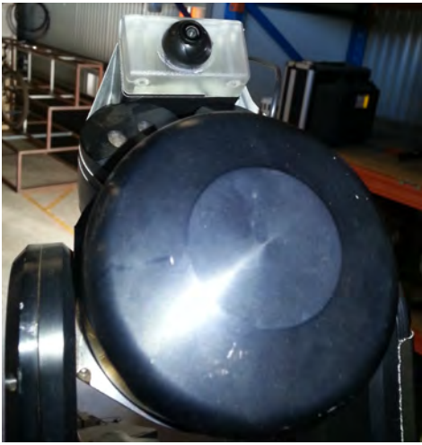
Fig. 3. The wide angle camera attached to the back of one of the existing pan-tilt-zoom cameras.
